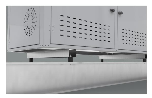
The rubber cylinder has been selected for optimum vibration absorption, with a hardness rating of 55 Shore A, specially selected for the application range. The mounts can be used for smaller machines with maximum compressive loads from under 4kg and a deflection of 0.9mm, up to heavy loads over 190kg with a deflection of 3.2mm. The smallest mounts have a cylinder length of just 8mm, while the largest extend to 30mm.
