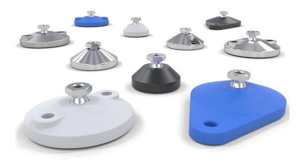
A compact, swivel ball insert provides 50° forward and backwards tilt across a 360° horizontal plane, enabling the feet to adjust to unlevel floors or uneven ground. Based on our extensive range of male insert self-levelling feet, the new design uses a compact, female thread insert instead of the extended male thread. This gives the swivel feet a low profile, reducing the height of the machinery or installation.
